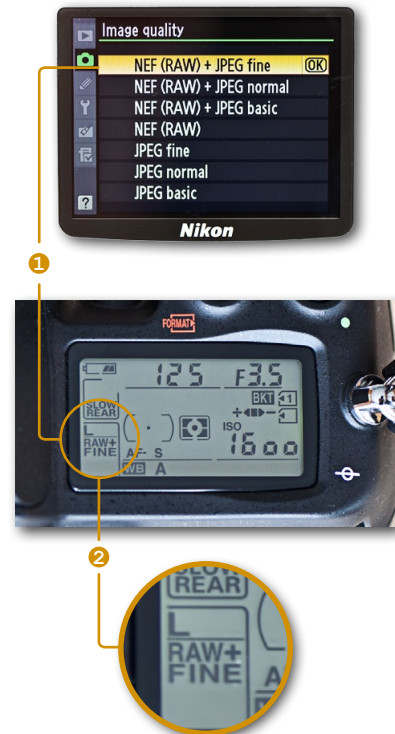
Figure 4 Activating RAW images on a Nikon camera. Activate them in the menu (1) and verify the correct setting on the display (2).
